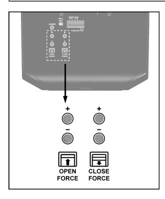
For safe operation, the force setting should always be set at the MINIMUM FORCE required to run the door.
